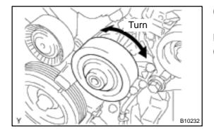
(b) Turn the pulley, and check that the water pump bearing moves smoothly and quietly.
